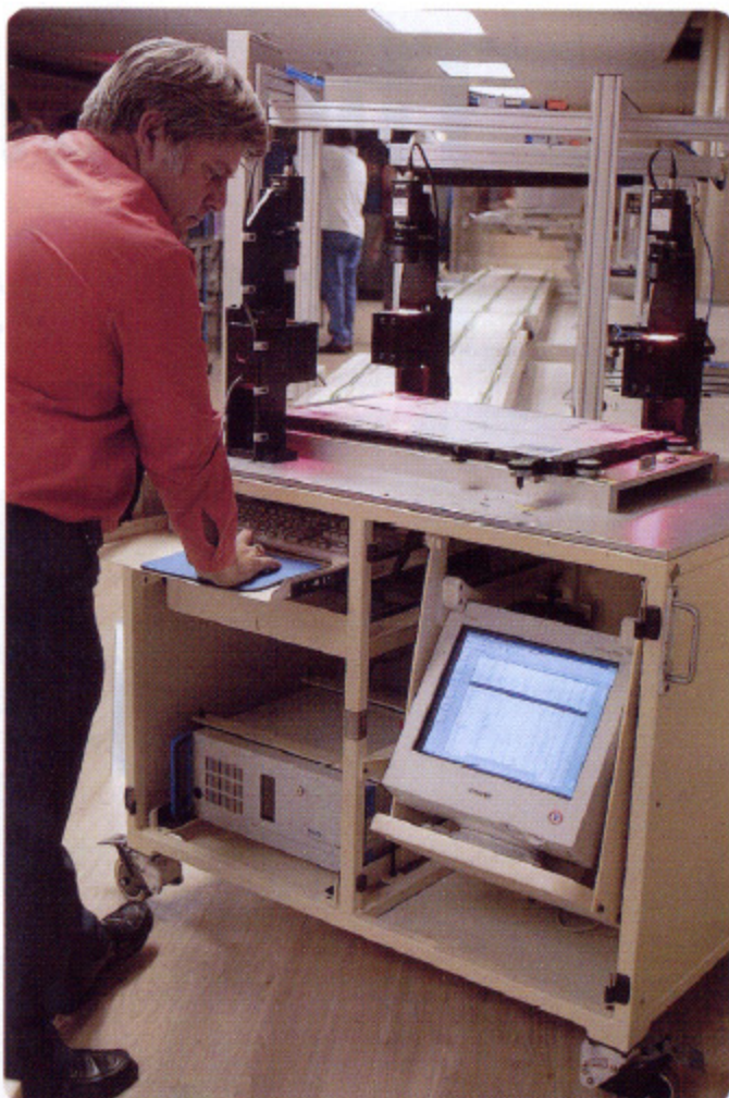
Print plate alignment checks at News International's Wapping plant are undertaken using Matsushita's P400 vision system
